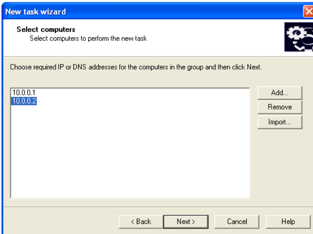
Figure 36. Creating the list of computers for installation based on IP addresses
